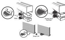
Wider shades have (2) Handles – to precisely determine the correct position for each handle, divide the total width of the shade by 4, and then attach one handle that distance from each outside edge of the shade – always grasp both handles when lifting and lowering the shade. For TDBU and Day/Night cordless shades, attach the 2nd handle to the Middle Rail as illustrated.
