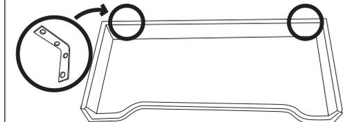
One bracket should be positioned about 6" from each end of the board. For wider shades that require up to 7 brackets, these should be spaced evenly between the two outermost brackets.
